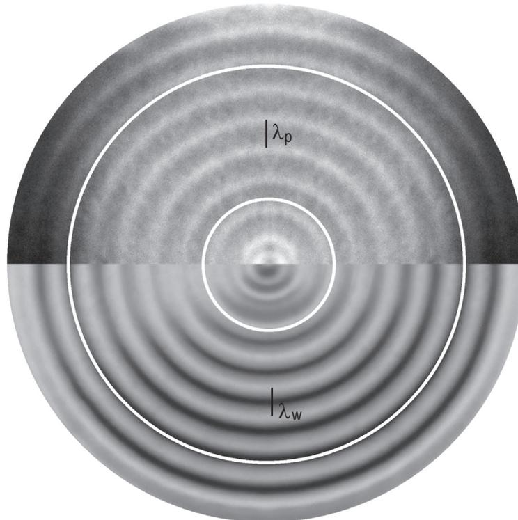
**Fig. 4.** Upper half: Patterned bed at steady-state, ridges appear lighter and troughs darker. Lower half: the waves at the free surface as acquired by the beam-splitter. The white circles indicate the inner and outer limits of the ROI, while the characteristic lengthscale of the patterned bed  $\lambda_p$  (given by the ridge-to-ridge distance), and wavelength of the surface waves  $\lambda_w$  are shown by short vertical bars. For both figures:  $f = 65$  Hz,  $\Gamma = 1.03$ , sample N° 2.
